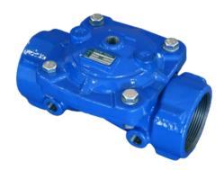
The FLUM VALVES cast iron hydraulic valve is a SANDERS type diaphragm hydraulic valve with a single chamber, with a basic opening and closing operation due to the pressure exerted by the water in the pipeline.
