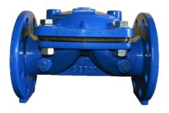
The FLUM VALVES cast iron hydraulic valve is a SANDERS type diaphragm hydraulic valve with a single chamber, with a basic opening and closing operation due to the pressure exerted by the water in the pipeline.
