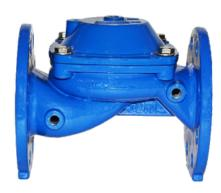
The FLUM VALVES HR-30 cast iron hydraulic valve is a diaphragm hydraulic valve with a vulcanized disc, with a basic opening and closing operation due to the pressure exerted by the water in the pipeline.
